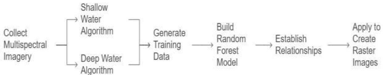
7-Fig: Flowchart for Water Temperature and Turbidity Retrieval Process
