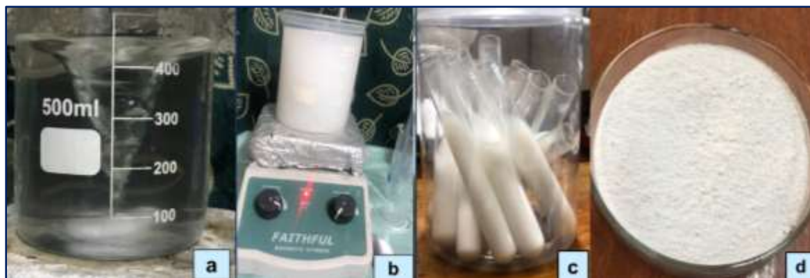
Figure 2. Preparation stages of 46S19 bioactive glass by the sol-gel method: (a) sol formation, (b) gel formation, (c) dried gel, and (d) calcined bioactive glass powder
