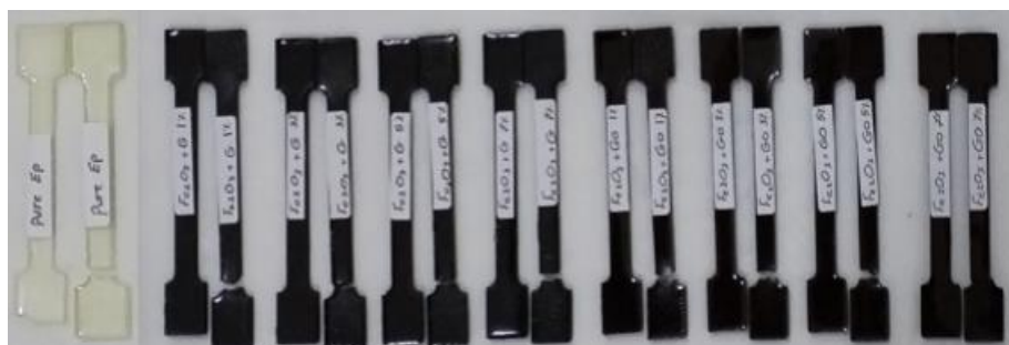
Figure 1: Tensile test specimens of epoxy nanocomposites.
