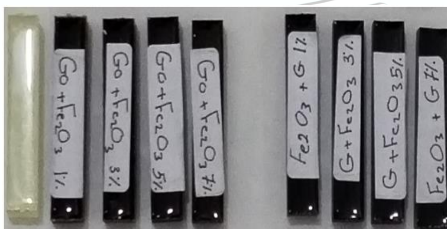
Figure 4: Charpy impact test specimens of epoxy nanocomposites reinforced with Fe 2 O 3 nanoparticles, graphene (G), and graphene oxide (GO) at different weight fractions.
