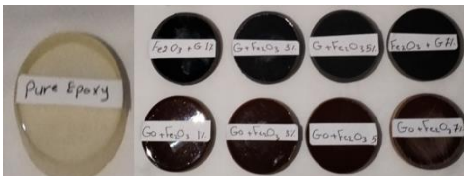
Figure 5: Shore D hardness test specimens of epoxy-based nanocomposites.
